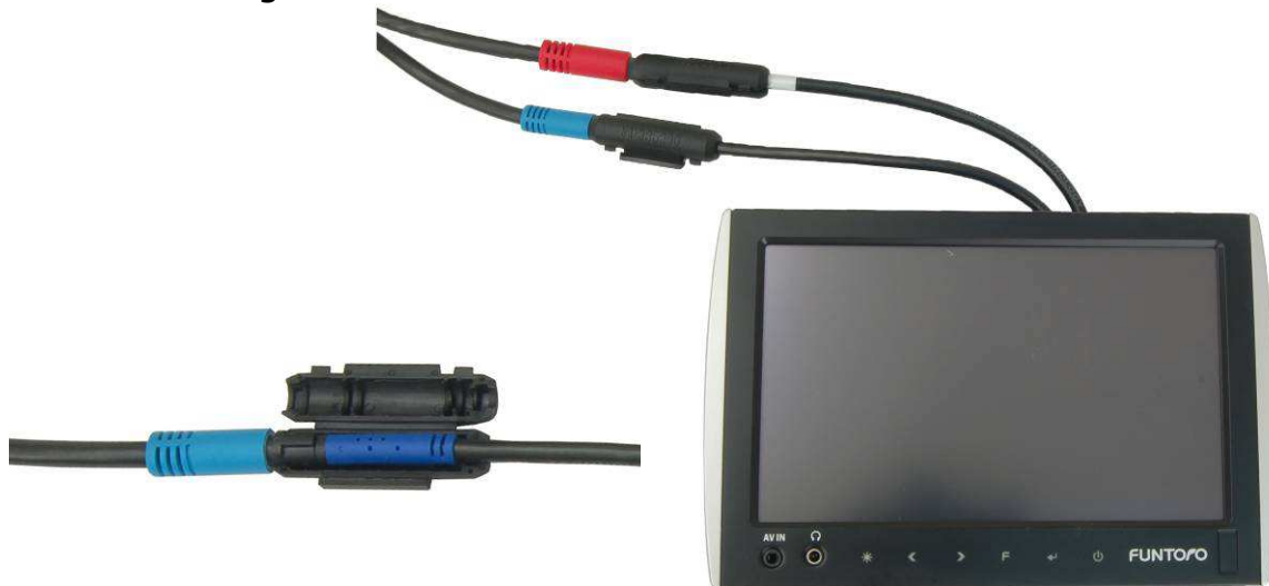
Figure 5 - AUX-IN and SPK-OUT cabling
