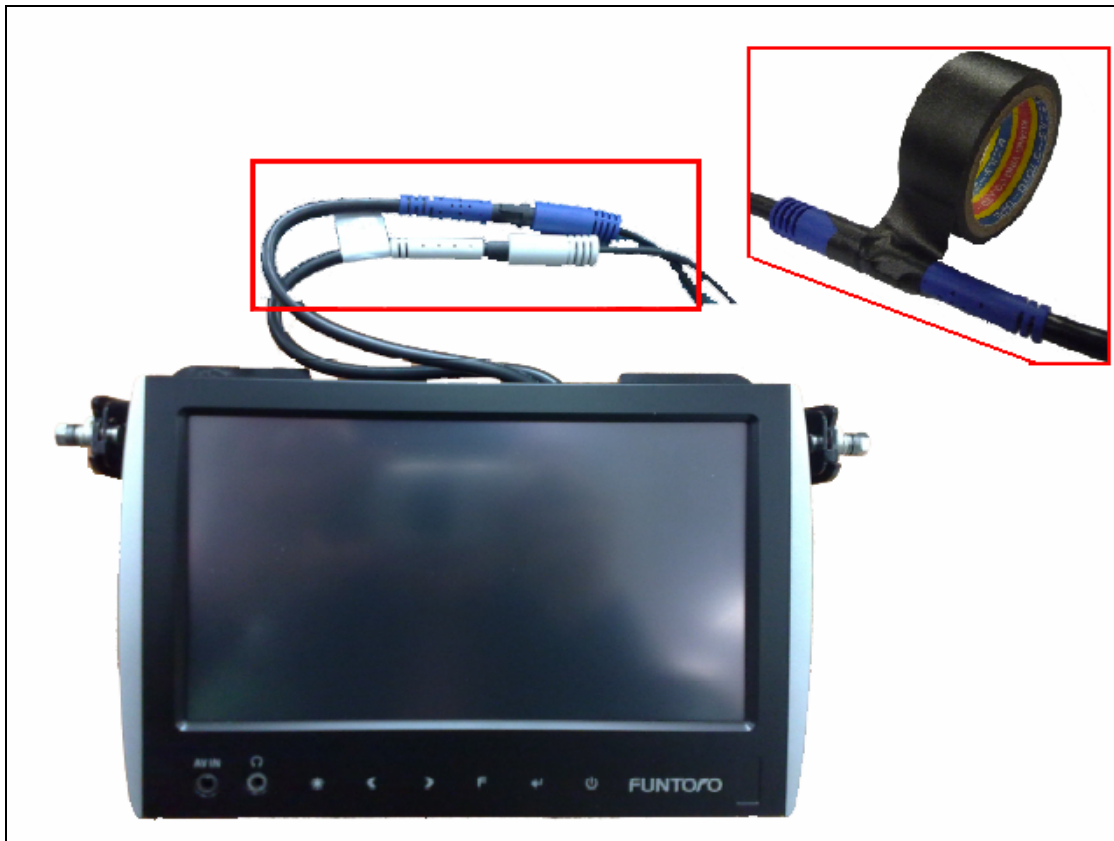
Figure 10, AUX-IN and SPK-OUT connection.
