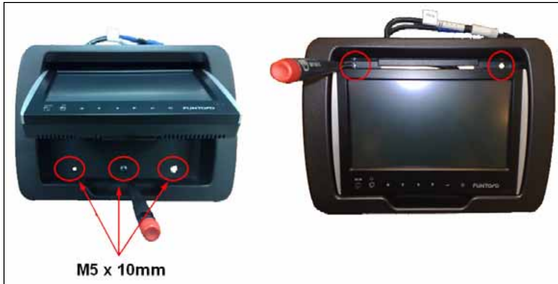
Figure 12, fit holder by screws.
